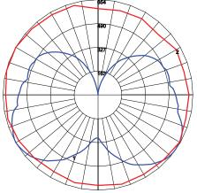
Maximum Candela = 653.621 Located At Horizontal Angle = 150, Vertical Angle = 6 # 1 - Vertical Plane Through Horizontal Angles (150 - 330) (Through Max. Cd.)
