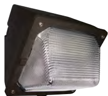
Small Wall Pack AIWP12Q 18-28 Input Watts; 2,000-3,200 Lumens Replaces up to 100w HID
