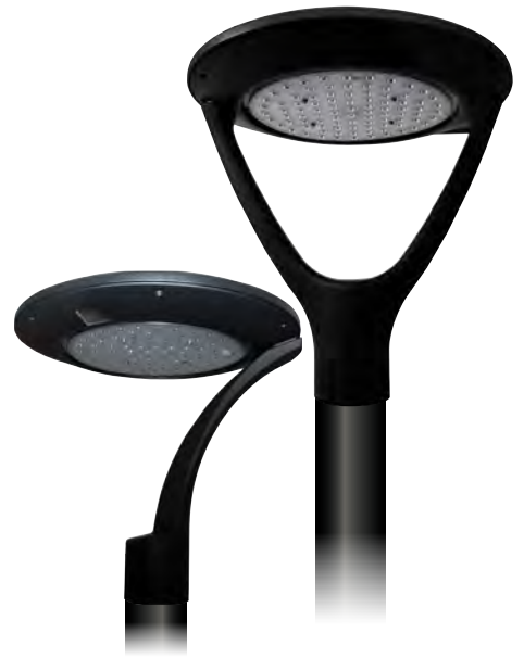
Allora II Round Post Tops AIAFR31Q & AIAFR32Q 41-156 Input Watts; 4,600-19,500 Lumens Replaces up to 400w HID
